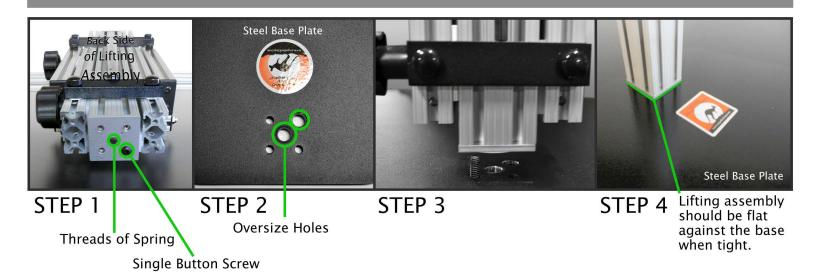
Step 1: Lay the lifting assembly on a solid surface with the back side up as shown. Notice the single Button Head Bolt and the Threads of the Spring in the assembly union. DO NOT LOOSEN THE SINGLE BUTTON HEAD BOLT.
