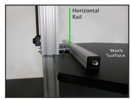
Step 8: Lift the Work Surface up and align the holes in the Horizontal Rail with the (2)  $1/4-20 \times 3.50$  Hex Head Bolts. Push the Work Surface onto the Hex Head Bolts until the threads of the bolts come through the Horizontal Rail.
