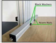
Step 9: Put (1) Black Washer and (1) Acorn Nut on the end of each of the Hex Head Bolts. Using the 7/16 wrench, tighten the Acorn Nuts securely.
