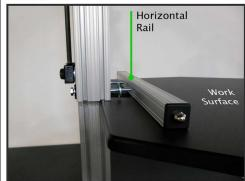
Step 8: Lift the Work Surface up and align the holes in the Horizontal Rail with the (2) 1/4-20 x 3.50 Hex Head Bolts. Push the Work Surface onto the Hex Head Bolts until the threads of the bolts come through the Horizontal Rail.
