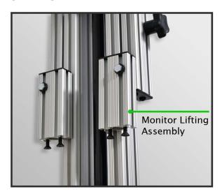
Step 5: Loosen both brakes and bring the unit to its full height. Re-tighten the brakes to hold position. Remove the (4) 1/4-20 x 1.0 flat head bolts from the bottom of the Monitor Lifting Assembly.
